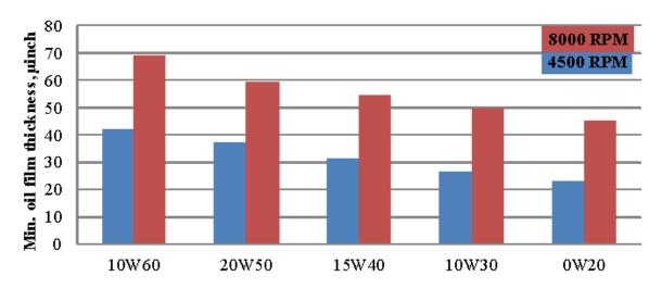
Changing from 10w60 oil to low viscosity 0w20 results in a 40% reduction of power loss in the bearing. In addition to friction reduction, low viscosity oils cling less to the connecting rod surface, thus reducing effective rod weight. Since connecting rods perform accelerating (reciprocating) movement, the power required for the inertia forces is proportional to the rod weight. With less oil adhering to the rod surfaces, less power is required for their movement.
