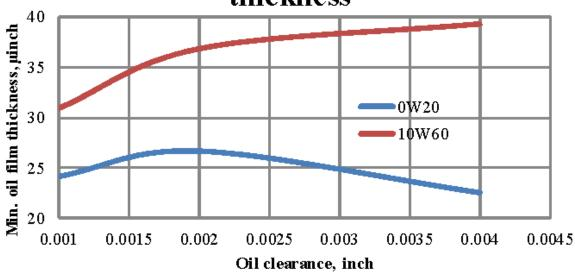
A low viscosity oil can maintain stable hydrodynamic lubrication between the bearings and crank journals with relatively low oil clearance (below 0.0025"). However, "thick" oil works better with clearances exceeding 0.0025".
